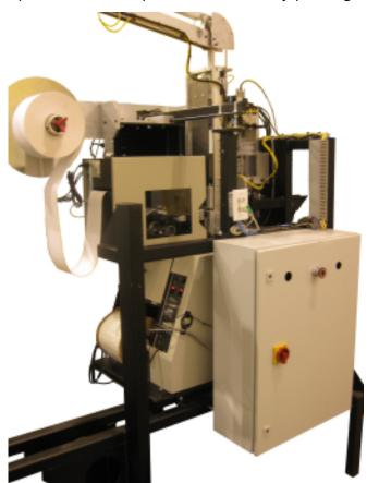
Incorporated into this unit is a five inch wide direct thermal printer and folding mechanism capable of handling 12 inches per second and up to thirty nine inches in length of print.
